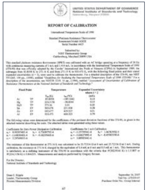
Example of Thermometer Certificate of Traceability and Calibration Testing (also known as a Report of Calibration). This could be a multiple page document.
