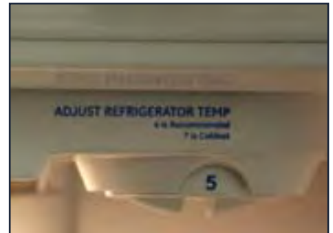
Refrigerator unit thermostat
