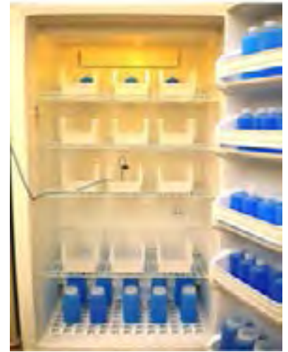
Probe in glycol bottle is placed in proximity to vaccines
