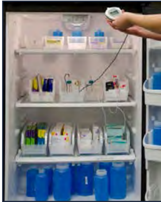
Digital thermometer with probe in glycol-filled bottle
