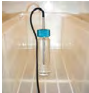
Probe in glycol bottle inside unit is attached by cable to main monitor
